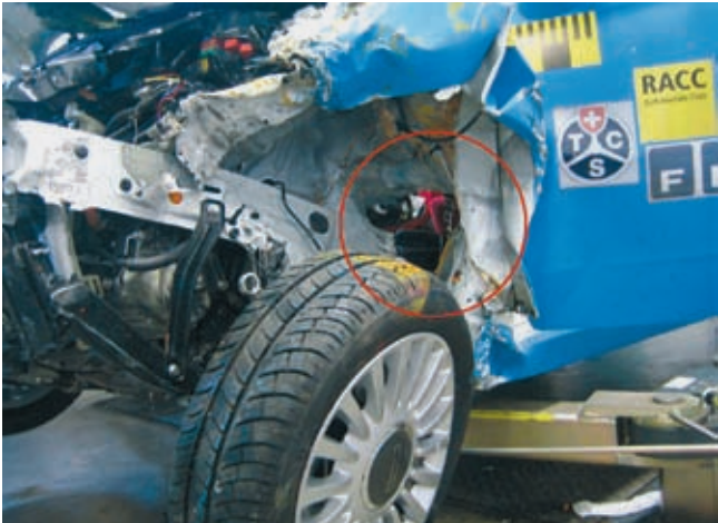
Figure 7: Hole in the Fiat's footwell
