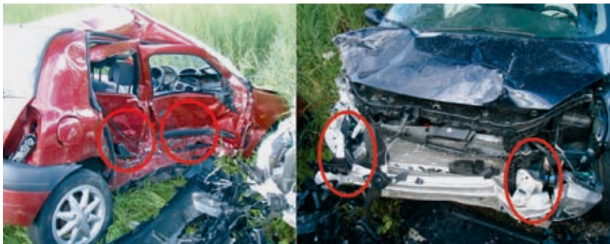
Figure 1: Incompatibility in a real-world side crash (ADAC accident research)
