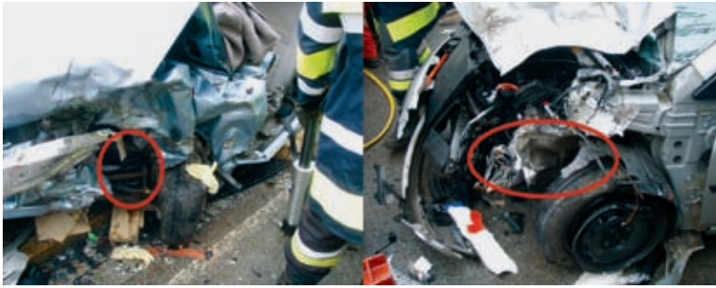
Figure 2: Incompatibility in a real-world frontal crash (ADAC accident research)
