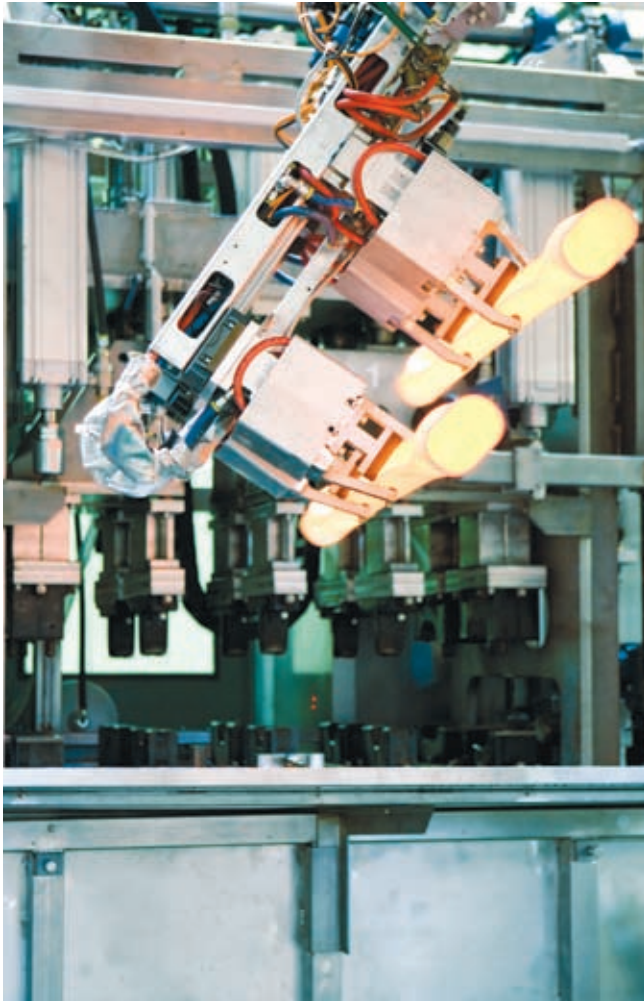
Figure 5: Twist beam made of steel BTR165 before water quenching
